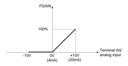
Figure 4.4.38 Frequency gain adjustment
