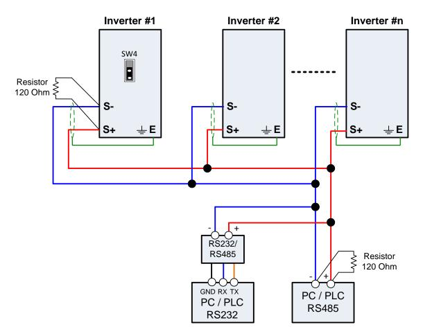
Wiring diagram RS485 Modbus RTU Network
