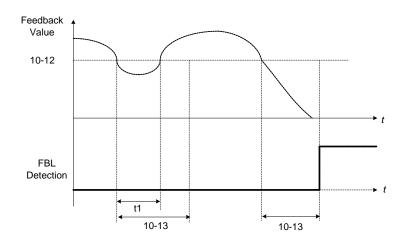
Figure 4.4.82 PID feedback loss detection
