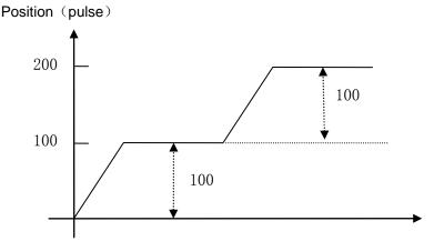
Figure 4.4.132 the absolute type diagram
