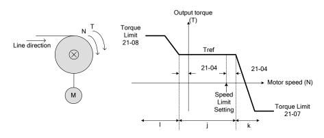
Figure 4.4.124 Winding operation
