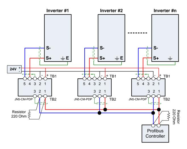
Wiring diagram Profibus DP Network
