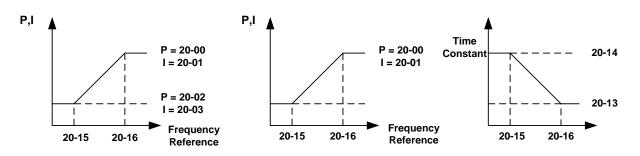
Figure 4.4.112 ASR gain setting (SLV mode)
