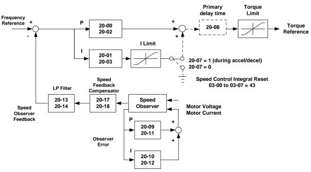
Figure 4.4.108 ASR block diagram (SLV mode)
