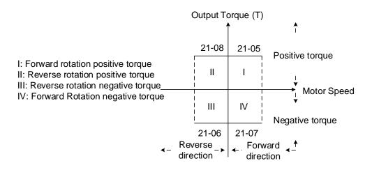
Figure 4.4.127 Torque limit setting
