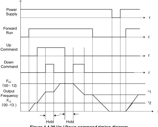
Figure 4.4.20 Up / Down command timing diagram
