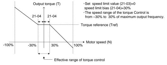
Figure 4.4.122 Speed limit setting
