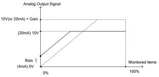
Figure 4.4.51 Analog output level adjustment
