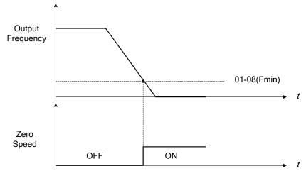
Figure 4.4.26 Zero-speed operation
