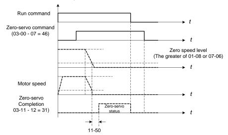
Figure 4.4.96 Zero servo operation
