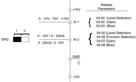
Figure 4.4.35 Analog inputs and related parameters
