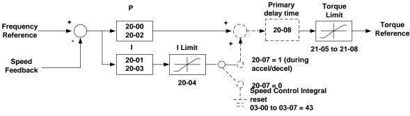
Figure 4.4.109 ASR block diagram (SV mode)
