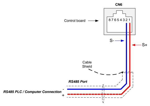
To control (Run/Stop) the inverter via serial communication parameter 00-02 has be set to either a "3" for communication control.
