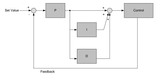
Figure 4.4.79 Basic PID control
