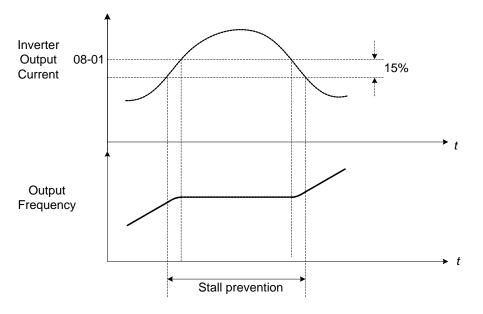
Figure 4.4.67 Stall prevention during acceleration
