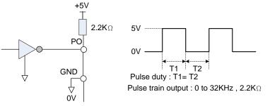
Figure 4.4.30 Pulse output signal level
