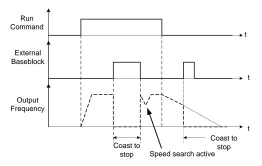
Figure 4.4.22 External base block operation
