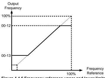
Figure 4.4.6 Frequency reference upper and lower limits
