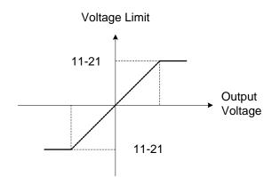
Figure 4.4.89 Voltage limit value of commissioning operation
