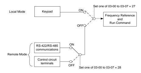
Figure 4.4.23 Remote mode operation selection
