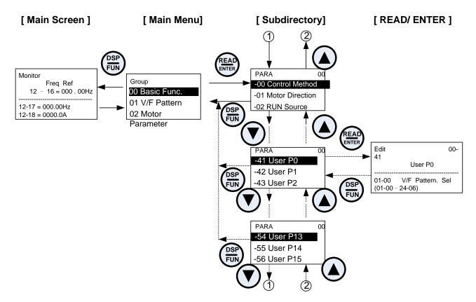
Note: User level (13-06=1) can be set by one or more parameters in the user parameters of 00-41 ~ 00-56.
