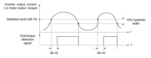
Figure 4.4.73 Over-torque detection operation
