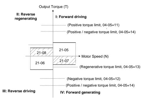
Figure 4.4.128 Analog input torque limit (Al2)
