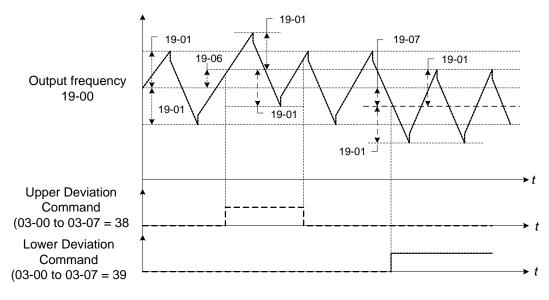
Figure 4.4.106 Upper/Lower offset operation
