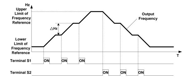
Mode 3: When 03-40 > 0 Hz and multi-function input terminals are active for more than 2 sec, frequency changes based upon acceleration / deceleration ramp.
