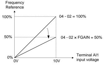
Figure 4.4.39 Frequency reference gain adjustment (example)
