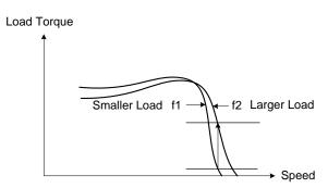
Figure 4.4.99 Slip compensation output frequency
