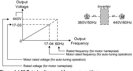
Figure 4.4.98 Rated voltage and frequency settings
