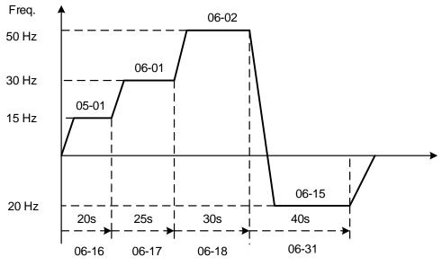
Figure 4.4.52 Single cycle automatic operation (stop)
