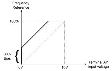
Figure 4.4.41 Frequency Reference bias adjustment (example)
