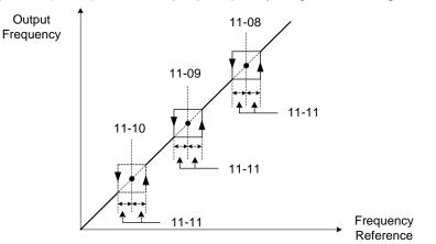
Figure 4.4.86 Jump frequency operation
