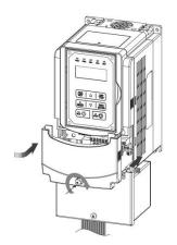
Step 5: Make connections and place filter cover back
