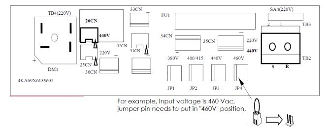
The inverter input voltage range of the A510 600V class models ranges from 575 to 690Vac. In these models the cooling fan is directly powered from the power supply. Inverter models A510s-6175~627 requires the user to select the correct jumper position based on the inverter input voltage ("690V" is the default position for these models). Please select the correct
