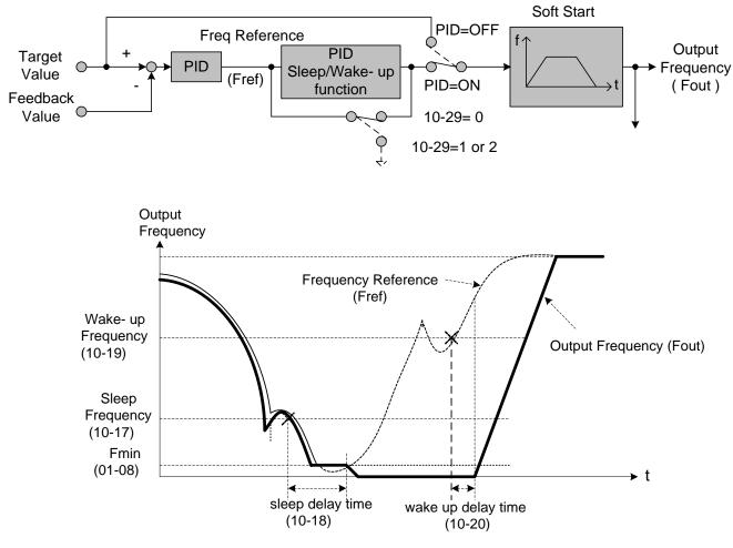
Fig. 4.4.83 PID Sleep Function
