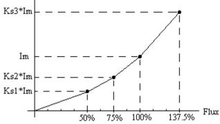
Im: 02-09 Excitation Current Ks1: 02-10 Motor Core Saturation Coefficients 1 Ks2: 02-11 Motor Core Saturation Coefficients 2 Ks3: 02-12 Motor Core Saturation Coefficients 3
