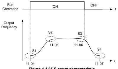
Figure 4.4.85 S curve characteristic
