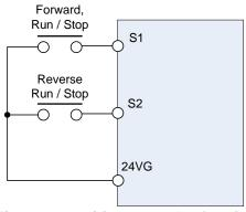
Figure 4.4.1 wiring example of 2-wire
