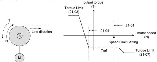
Figure 4.4.125 Unwind operation
