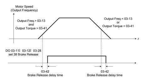
It is recommended to be with starting and stopping frequency locked function (11-43~11-46), shown as the following figure:
