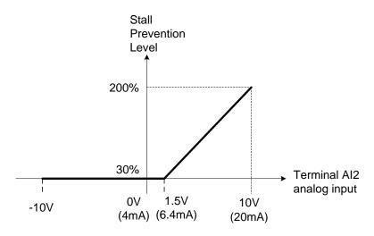
Figure 4.4.46 Stall prevention level adjustment in operation
