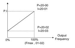
Figure 4.4.110 ASR gain setting (V/F+PG)
