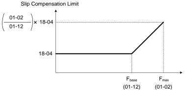
Figure 4.4.100 Slip compensation limit
