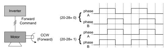
Figure 4.4.118 PG and motor rotation direction
