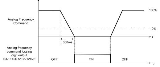
Figure 4.4.93 Operation in reference frequency loss
