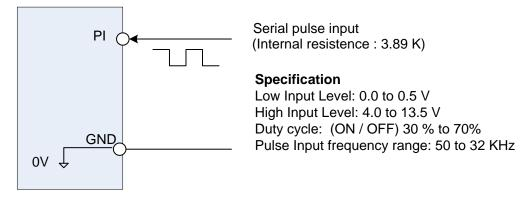
Figure 4.4.5 Frequency reference from pulse input
