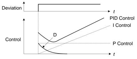
Figure 4.4.77 PID Control
