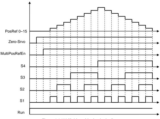
Figure 4.4.130 Multi-positioning logic diagram
