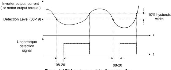
Figure 4.4.74 Low torque detection operation
