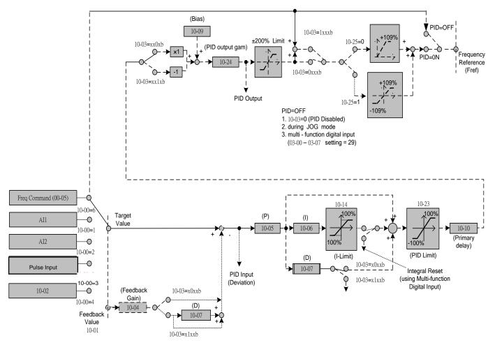
Figure 4.4.81 PID control block diagram
