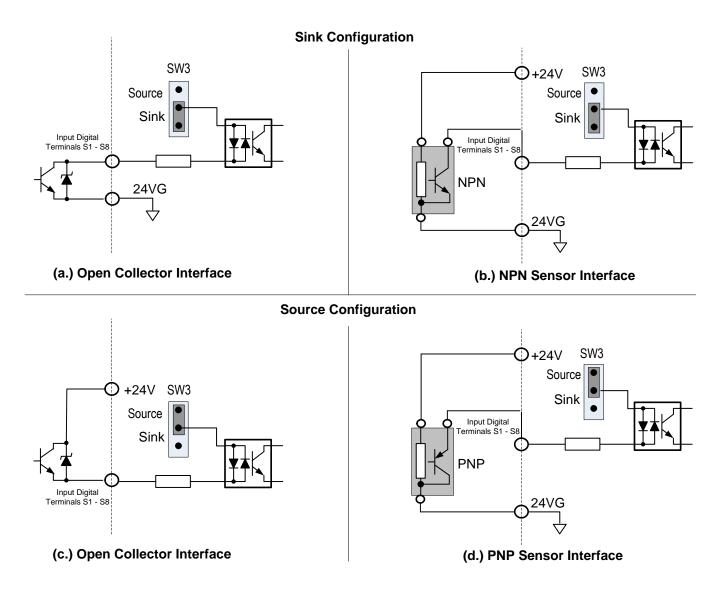
Fig. 3.17.3 Sink / Source Configurations
