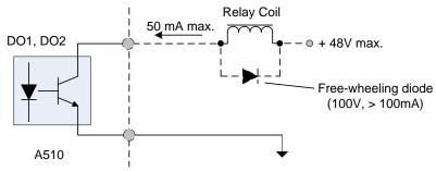
Fig. 3.17.2 Photo-Coupler Connected to an External Relay
