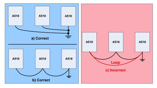
Fig. 3.12.1 Inverter Grounding
