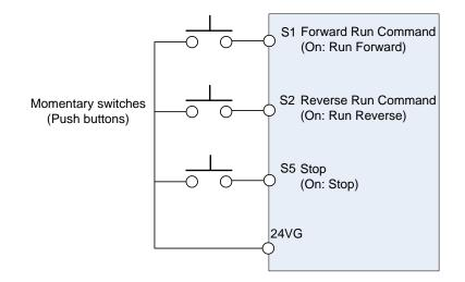
Note: Terminal S1, S2 and S5 must be closed for a minimum of 50ms to activate operation.
