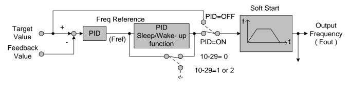
Figure 4.4.83: (a) PID control bock diagram
