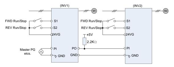
Figure 4.4.32 Speed follower using two inverters
