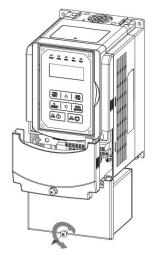
Step 3: Unscrew filter section
