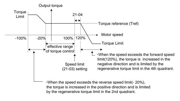
Figure 4.4.123 Speed limit setting (Example 2)
