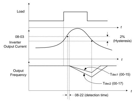
Figure 4.4.70 Stall prevention selection in operation
