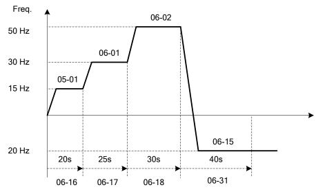
Figure 4.4.54 Single cycle automatic operation (continuous)
