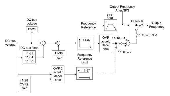
Figure 4.4.91 OVP operation
