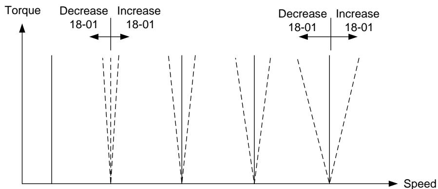
**Figure 4.4.103 18-01 Effect on torque speed curve**
