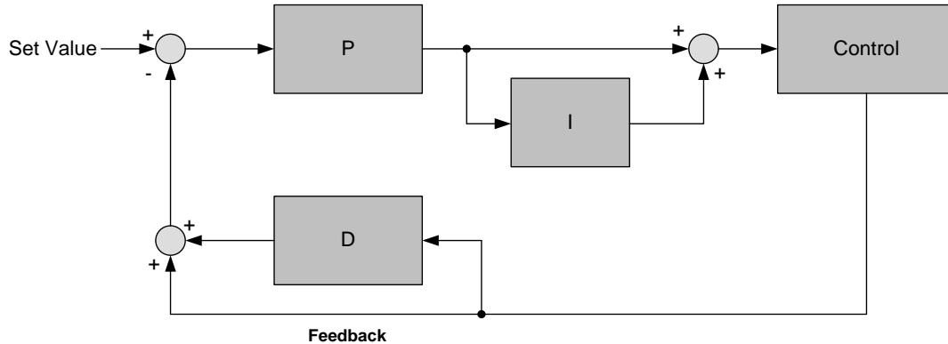
Figure 4.4.78 PID control for feedback differential value
