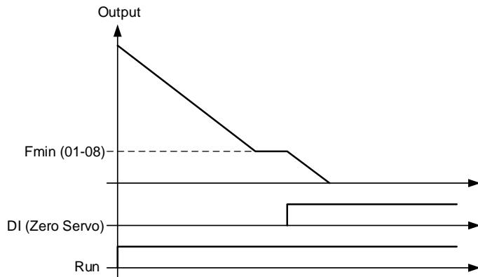
Figure 4.3.129 Zero-servo positioning
