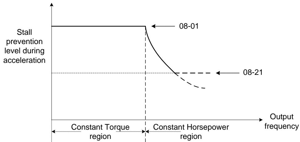
**Figure 4.4.68 Stall prevention level and limit in acceleration**
