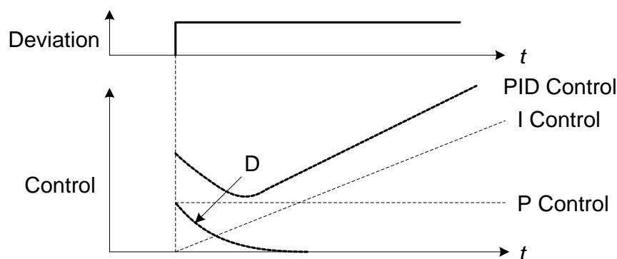
**Figure 4.4.77 PID Control**
