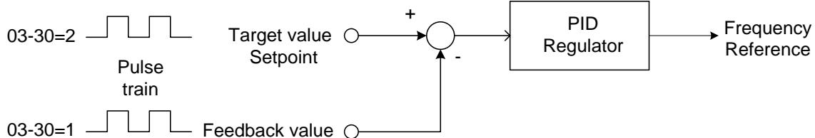
Figure 4.4.28 PID control
