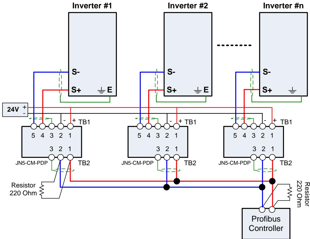
**Wiring diagram Profibus DP Network**
