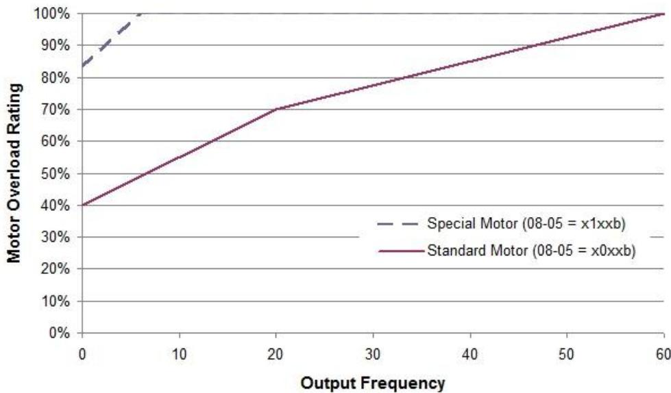
Figure 4.4.72 Motor overload rating at different output frequencies
