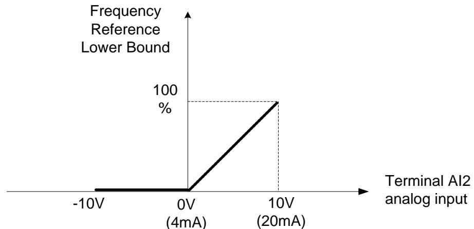
**Figure 4.4.47 Adjustment of lower limit of frequency reference**
