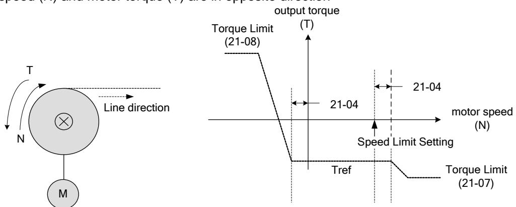
**Figure 4.4.125 Unwind operation**
