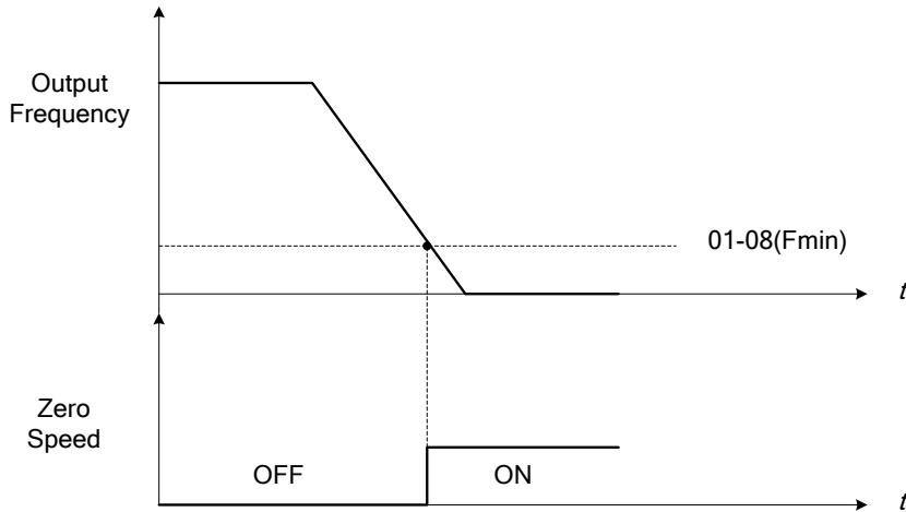
**Figure 4.4.26 Zero-speed operation**
