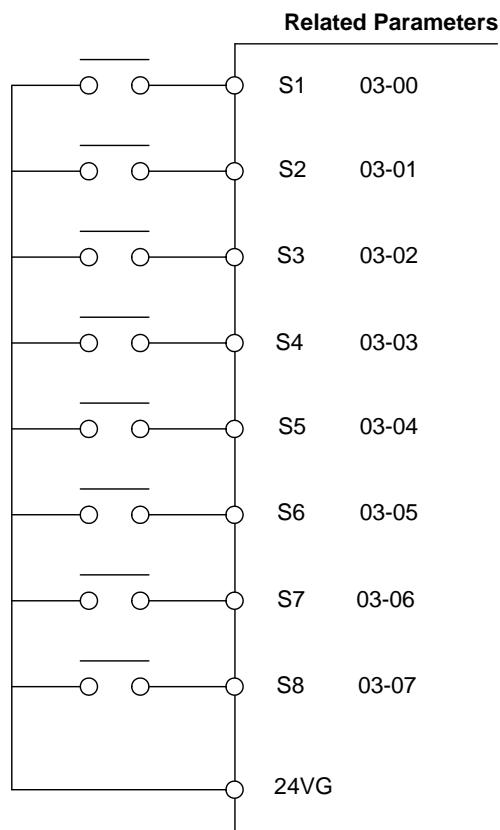
**Figure 4.4.16 Multi-function digital input and related parameters**
