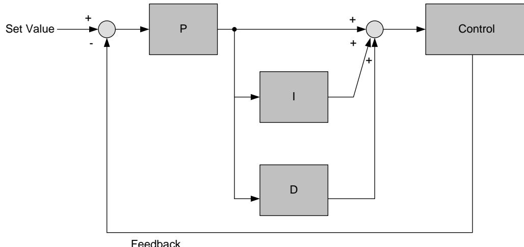
Figure 4.4.79 Basic PID control
