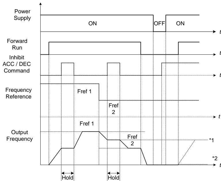
**Figure 4.4.21 Inhibit acceleration / deceleration command operation**
