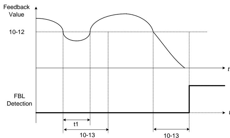
**Figure 4.4.82 PID feedback loss detection**
