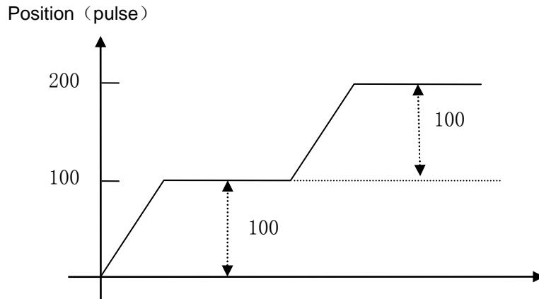
Figure 4.4.132 the absolute type diagram
