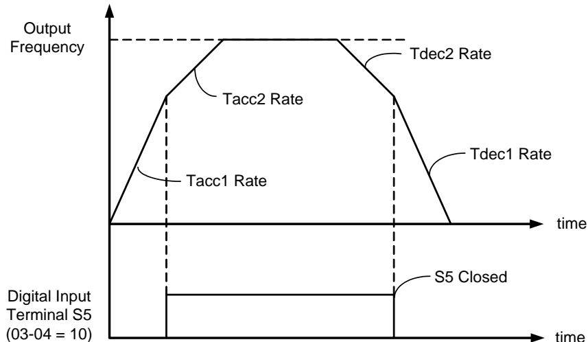
**Figure 4.4.7: Terminal S5 switch between Tacc1/Tacc2 and Tdec1/Tdec2**
