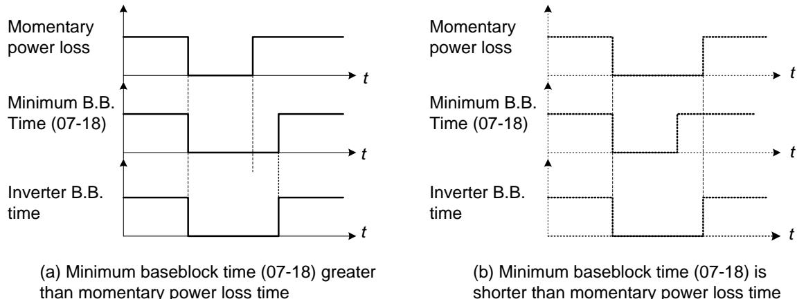
**Figure 4.4.63 Minimum B.B. time and momentary power loss time**
