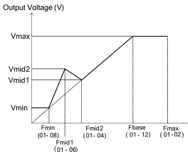
Figure 4.4.13 Torque boosting
