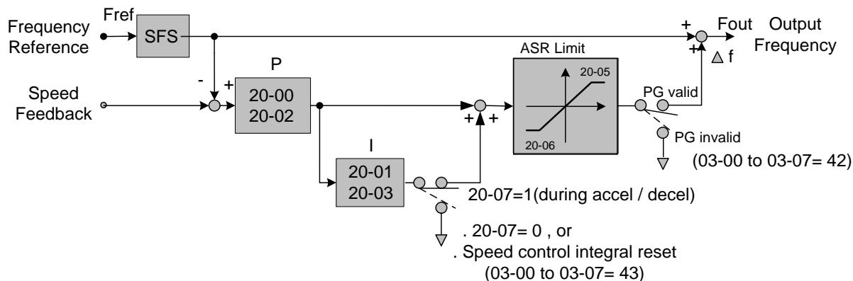
**Figure 4.4.107 ASR block diagram (V/F + PG)**
