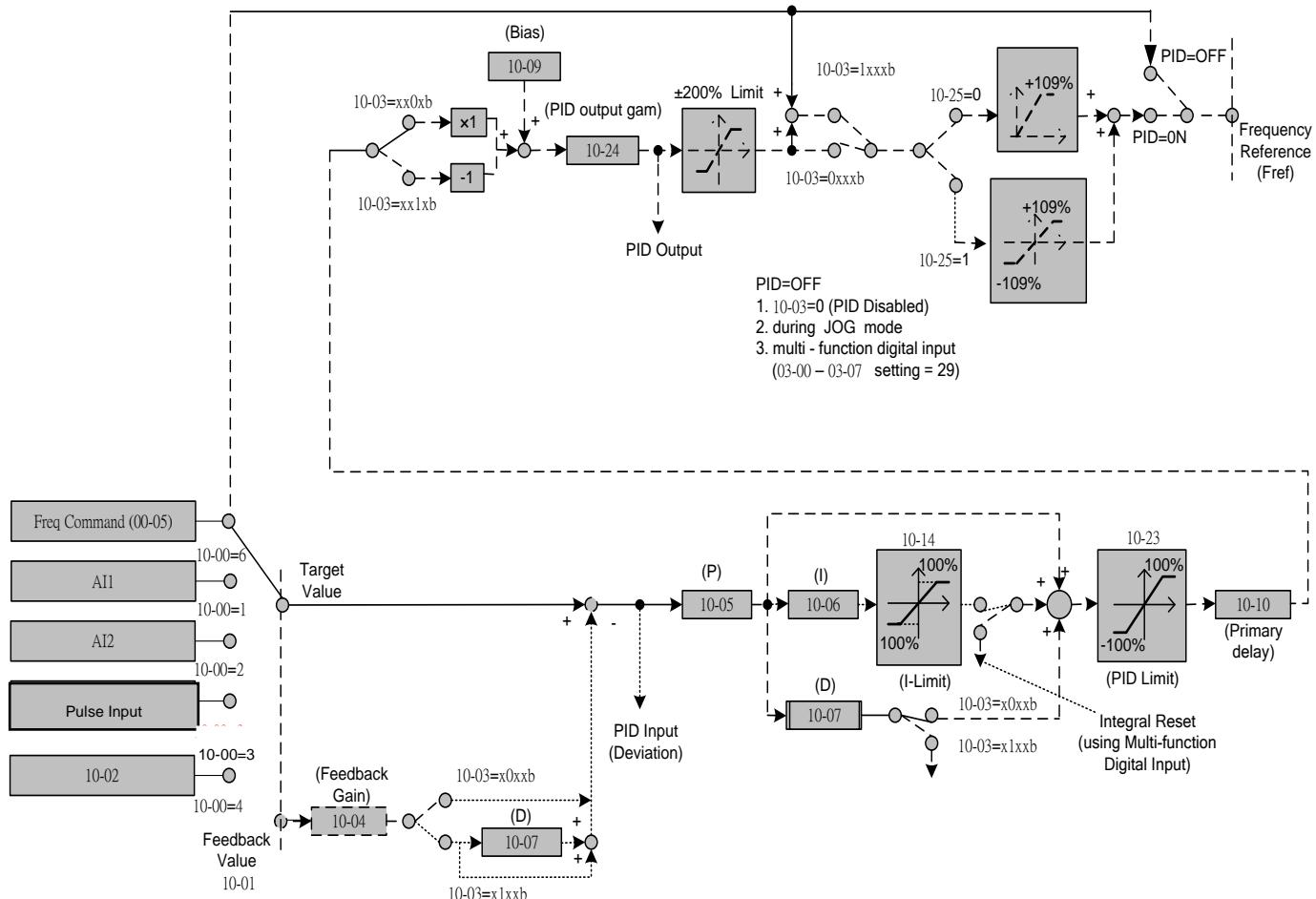
Figure 4.4.81 PID control block diagram
