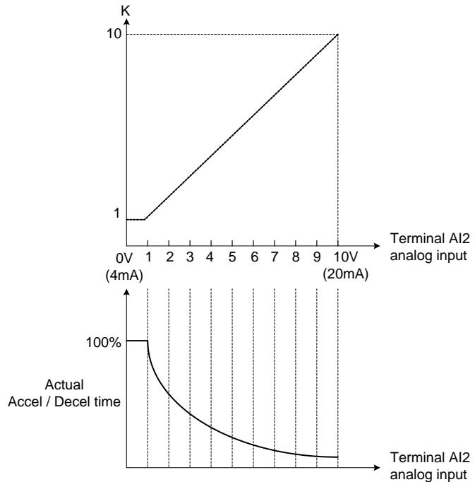
**Figure 4.4.43 Acceleration / deceleration time reduction coefficient**
