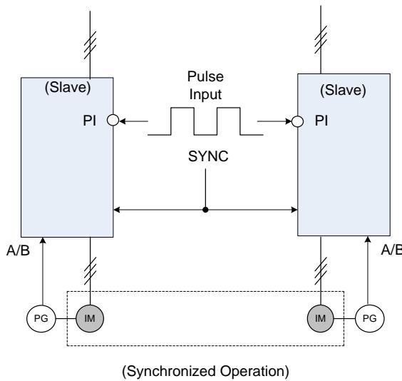
**Figure 4.4.33: Synchronized operation of using pulse input**
