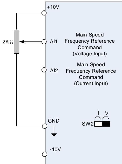
**Figure 4.4.4 Analog input as main frequency reference command**
