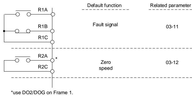
**Figure 4.4.25 Multi-function digital output and related parameters**
