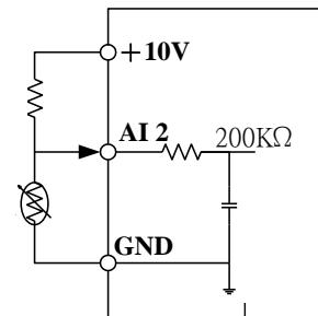
**Figure 4.3.65 (a) PTC Thermistor Characteristics (b) PTC Thermistor Connections**
