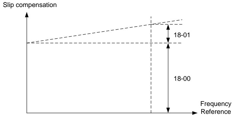
**Figure 4.4.102 18-00/18-01 Slip compensation gain versus frequency reference**
