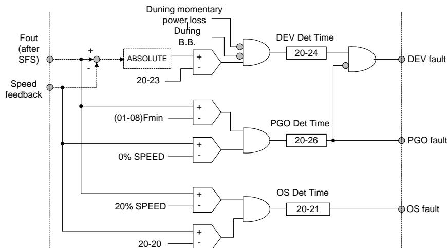
Figure 4.4.117 Logic diagram PG feedback failure detection
