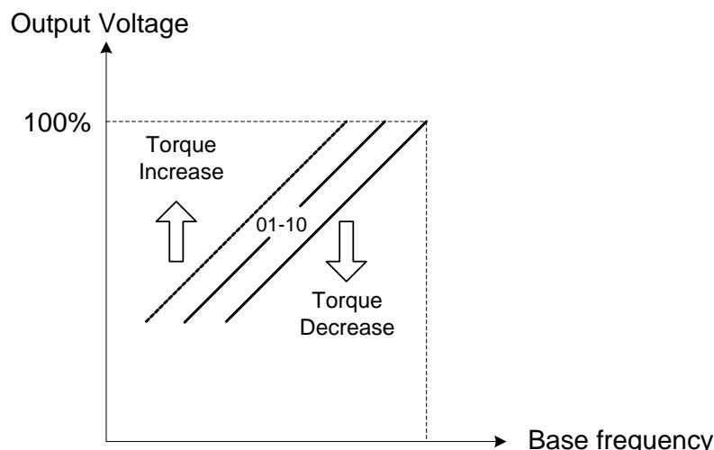
**Figure 4.4.14 Torque compensation gain to increase/decrease output torque**
