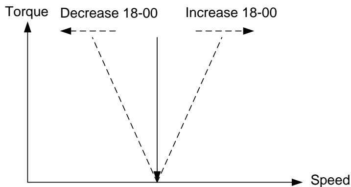
**Figure 4.4.101 18-00 Effect on the torque and speed**
