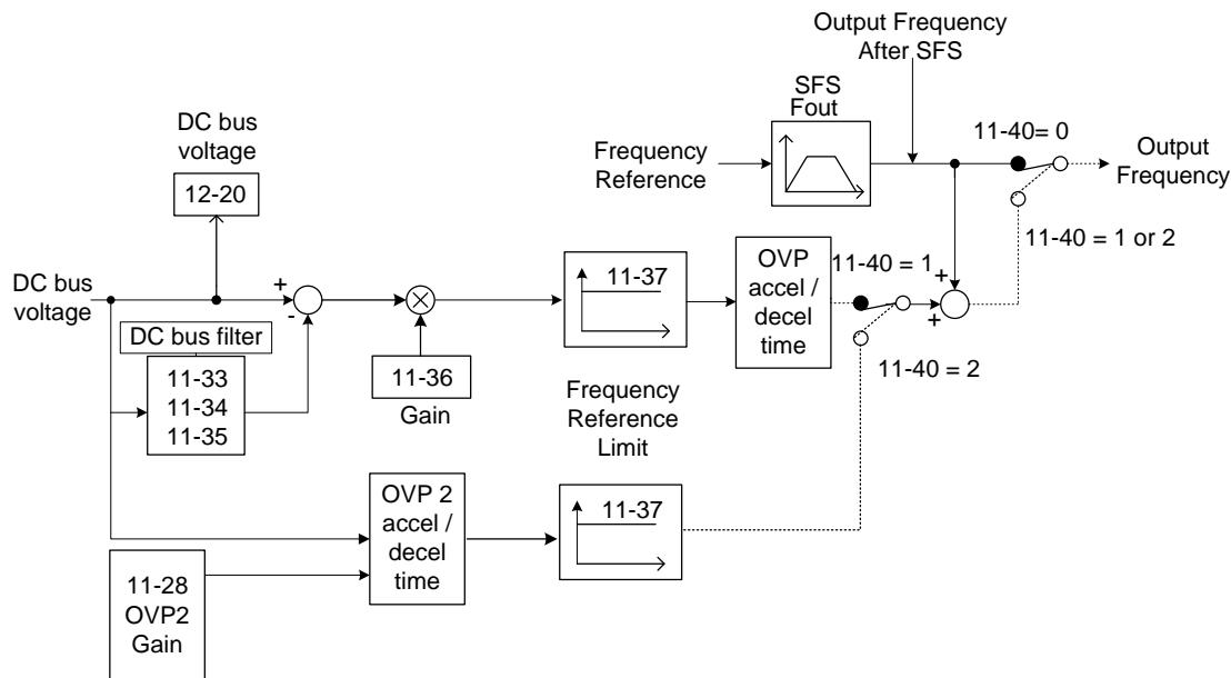
Figure 4.4.91 OVP operation
