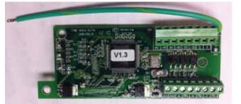
The A510 product has a standard RS485 port with RTU Modbus protocol. An optional card for Profibus Communications is available.
